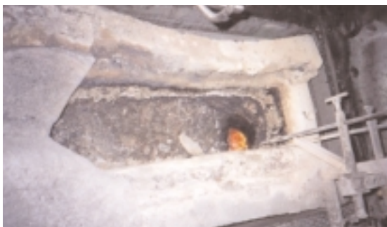
D-CAST TRC-SR-CC showing little signs of wear after 1 plus years of service in a pouring arm.
