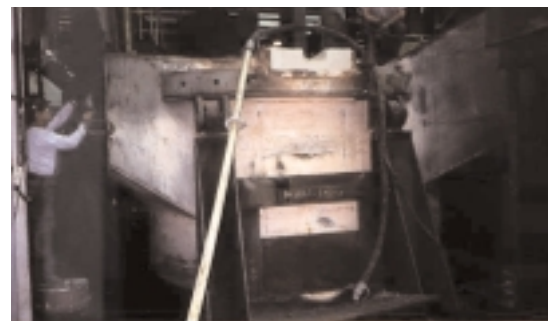
D-CAST TRC-SR-CC being pump cast into the pour spout and receiver.
