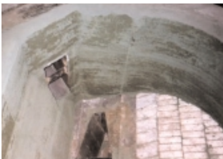
RUBY® RAMMING MIX lining the upper case and KORUNDAL XD® forming the jack arch and floor.
